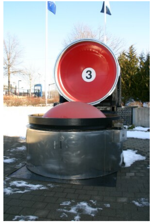
Missile launch tube. Upon launch the red cover comes off
