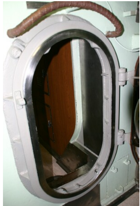
Passageway hatch - 18 inches from the floor
